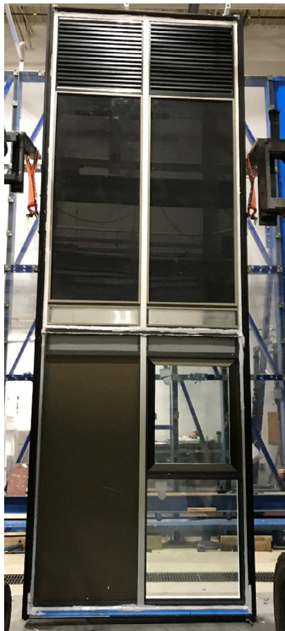
Photo 1: Window Wall Mock-Up
